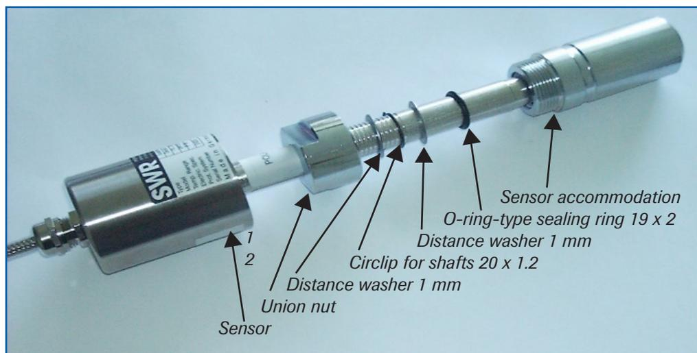
Fig. 5a: Installation of sensor accommodation and sensor
