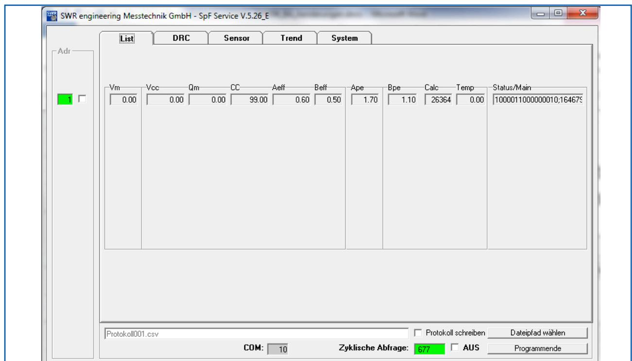
The sensor is portrayed with its main measurement value **Vm** and several secondary measurement values which provide information about the quality and condition of the measuring point.
