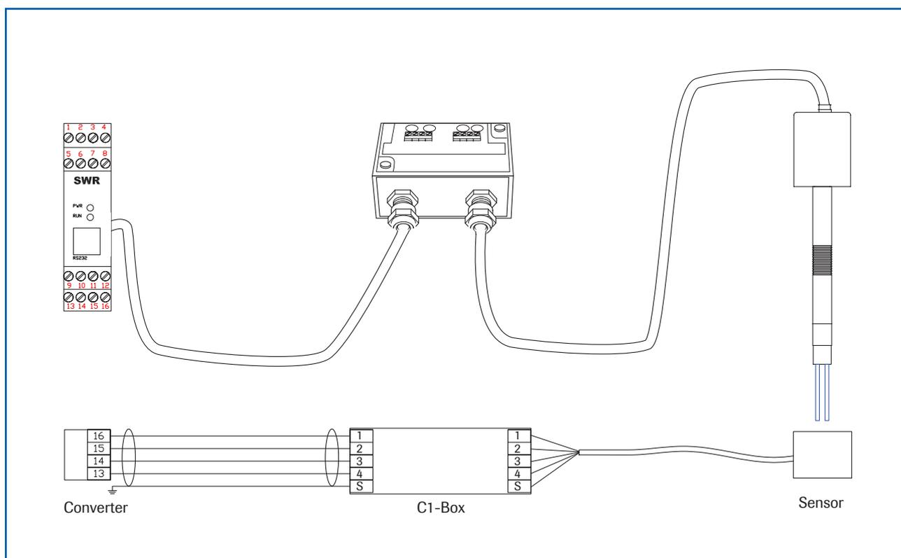
The measuring sensor is connected to the transmitter using a shielded 4-wired cable with the length of the cable not exceeding 300 m.
