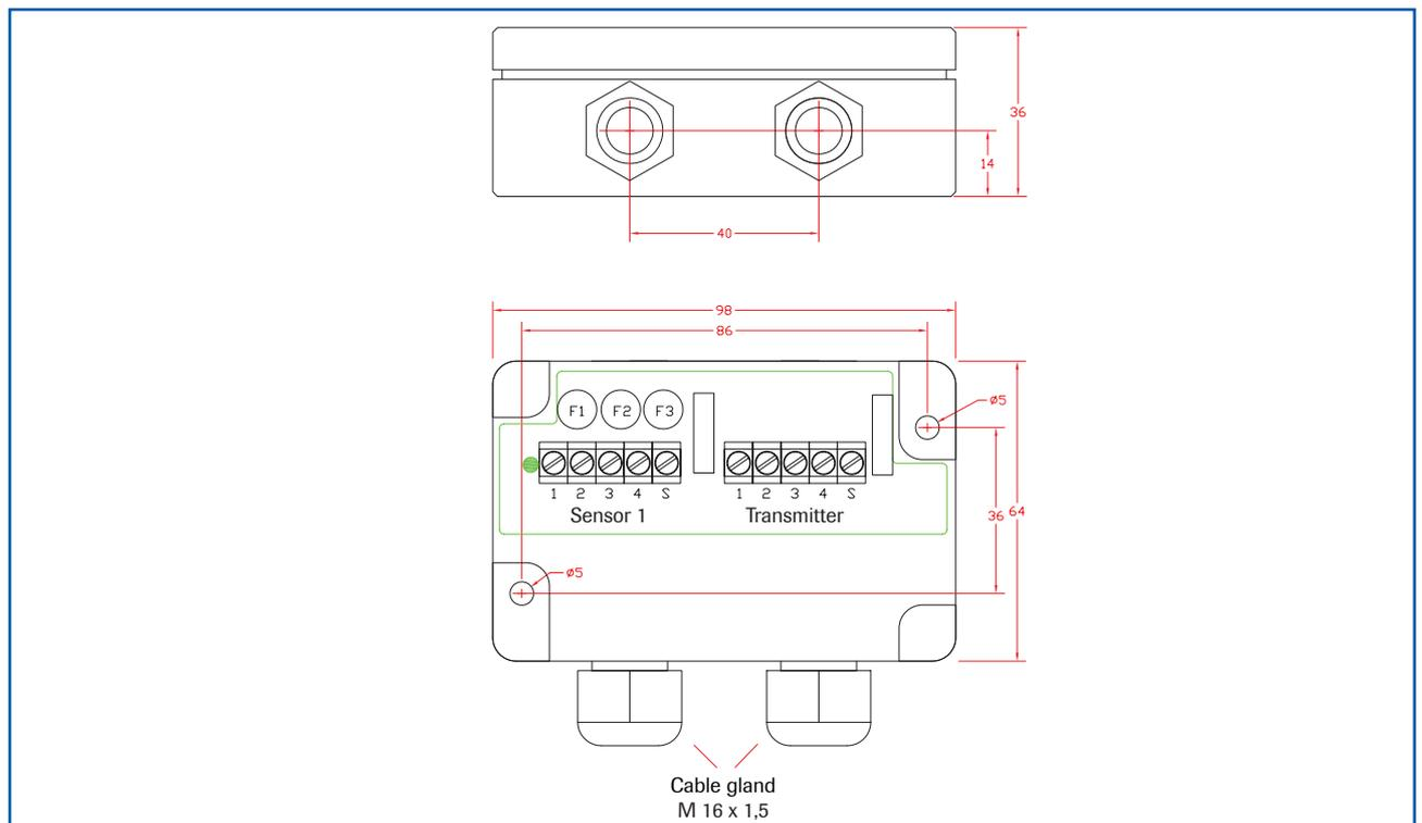
Fig. 7: Field housing for the C1-Box
