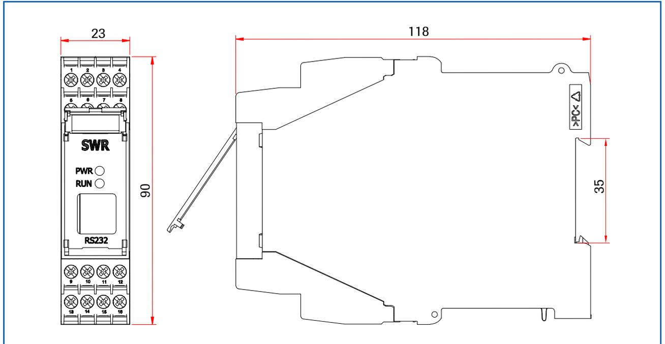
Fig. 6: DIN rail housing for the transmitter
