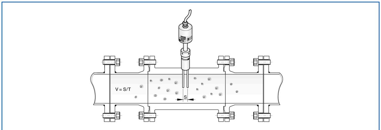
Fig. 2: SpeedFlow sensor in the pipeline
