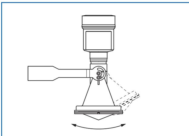
Fig. 8: Adjusting the tilt angle
