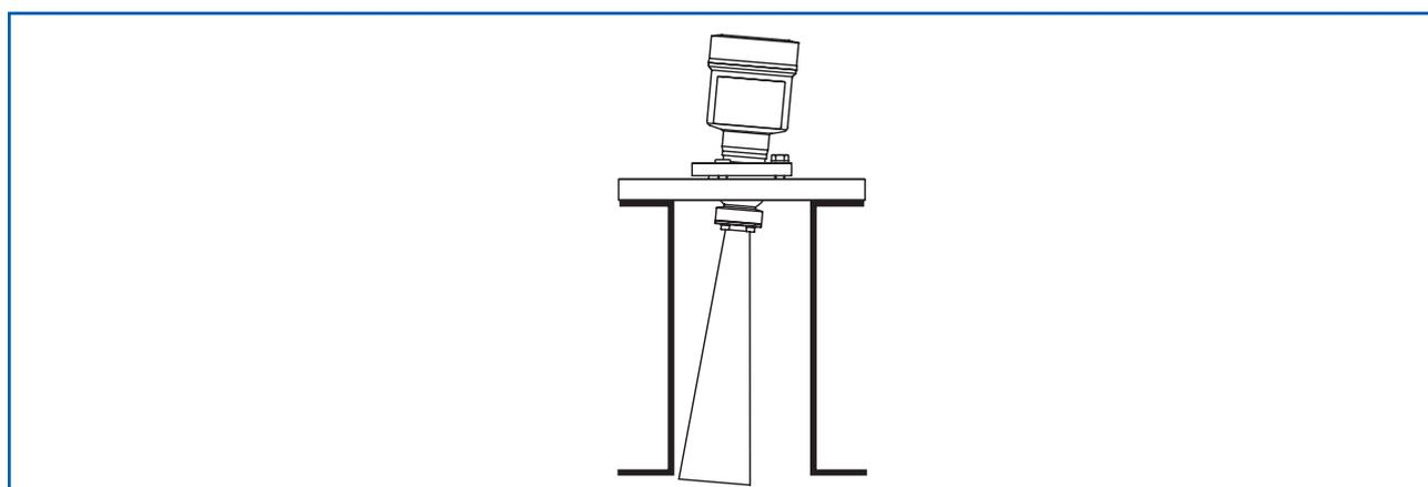
Fig. 17: Distance between the antenna and socket for horn antenna
