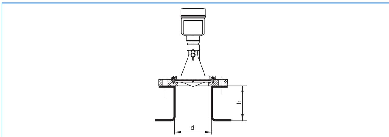
Fig. 15: Installation with a longer socket
