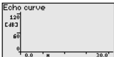
The "False signal suppression" represents the saved interference echoes (see "Additional adjustments" menu) for the empty vessel with the signal strength in "dB" over the measuring range.
