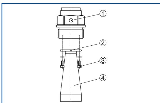
Fig. 4: Removing the horn antenna
