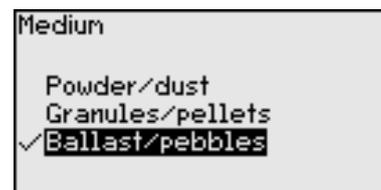
This selection will adjust the sensor perfectly to the product and significantly increase measurement accuracy, primarily for media with poor reflection properties.
