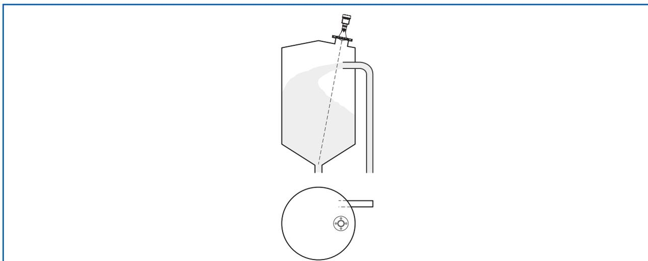
Fig. 13: Radar sensor installation with inflowing solids
