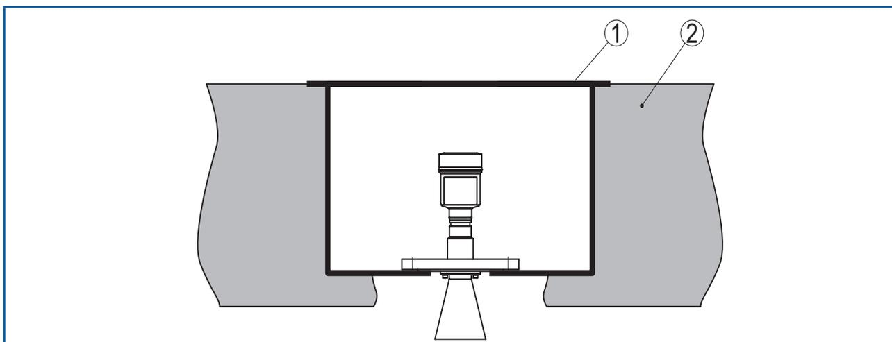
Fig. 25: Device installation in an underfloor box
