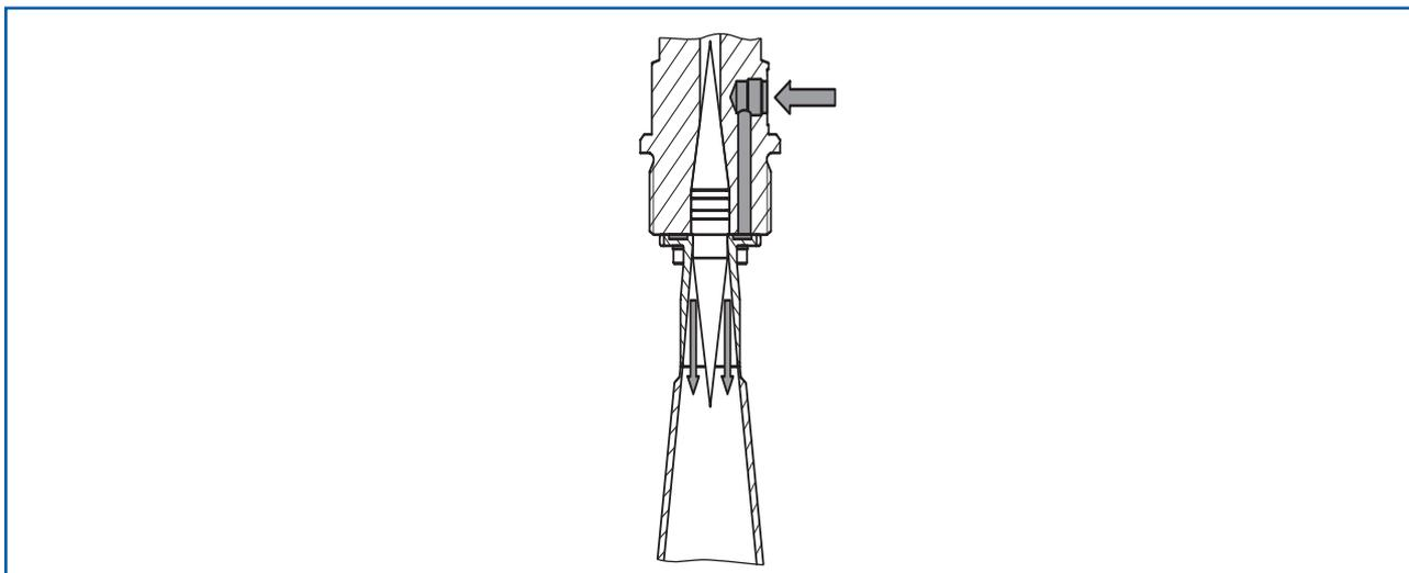
*Fig. 28: Purge air connection for horn antenna*
