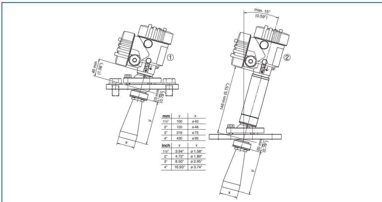
Fig. 42: Nico 30, horn antenna and swivel mounting
