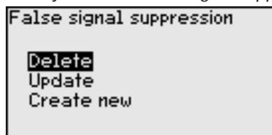
The "Delete" menu point can be used to delete a complete false signal suppression which has already been created. This is a good idea if the created false signal suppression no longer matches the measuring conditions in the vessel.
