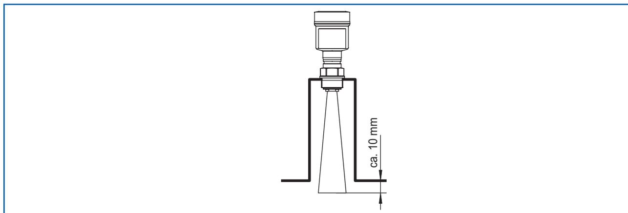
Fig. 16: Recommended pipe socket installation for horn antenna
