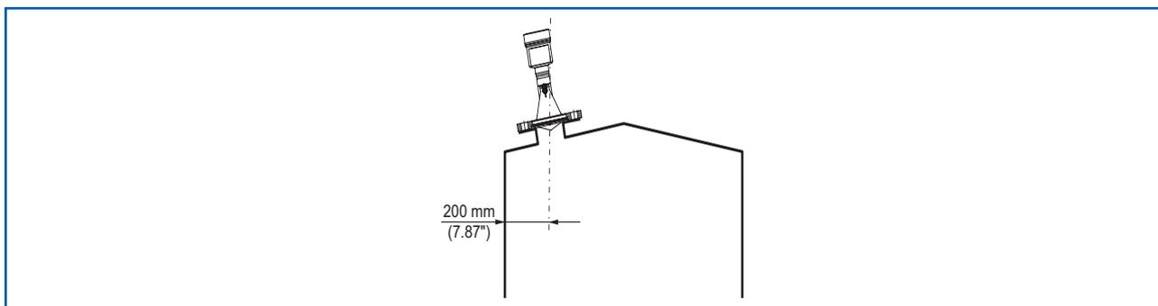
Fig. 6: Radar sensor installation in the vessel roof
