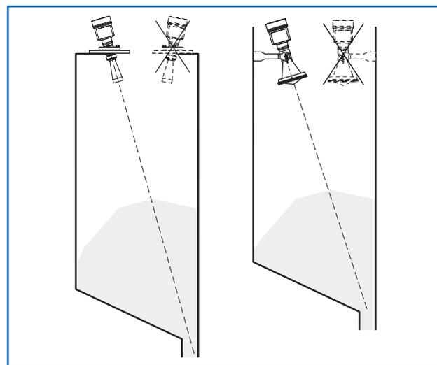
Fig. 27: Alignment to the discharge in the centre of the silo
