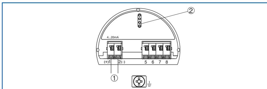
Fig. 2: Connection chamber for twin chamber housing for mains voltage
