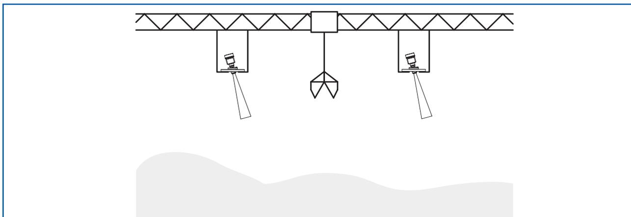
Fig. 23: Radar sensors on a crane beam
