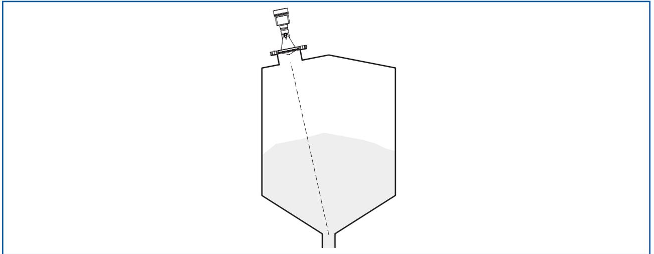
Fig. 10: Alignment in silos
