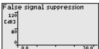
A comparison of the echo curve and false signal suppression enables a more precise assessment of the measurement reliability to be made. The selected curve is updated continuously. The **[OK]** key can be used to open a sub-menu with zoom functions:
