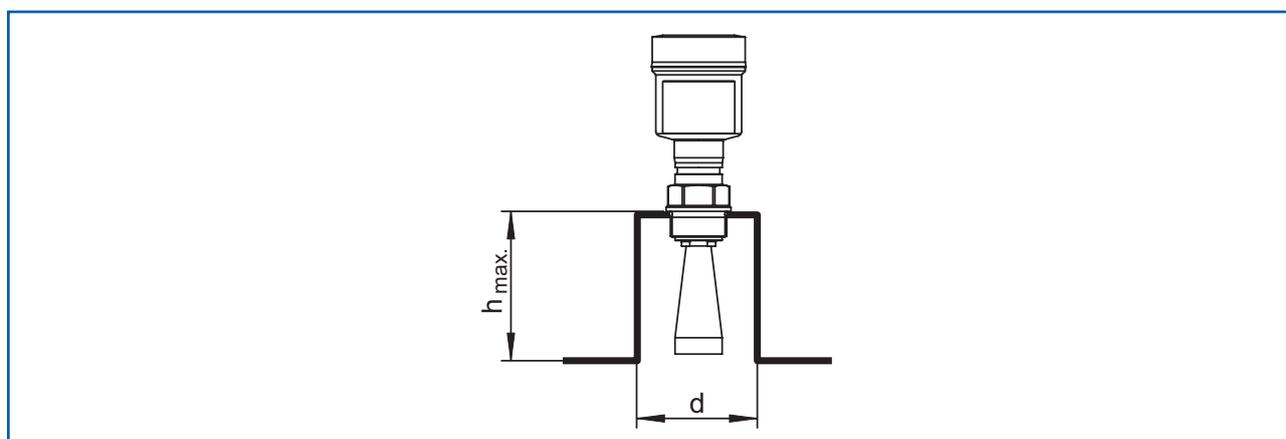
Fig. 18: Different pipe socket dimensions
