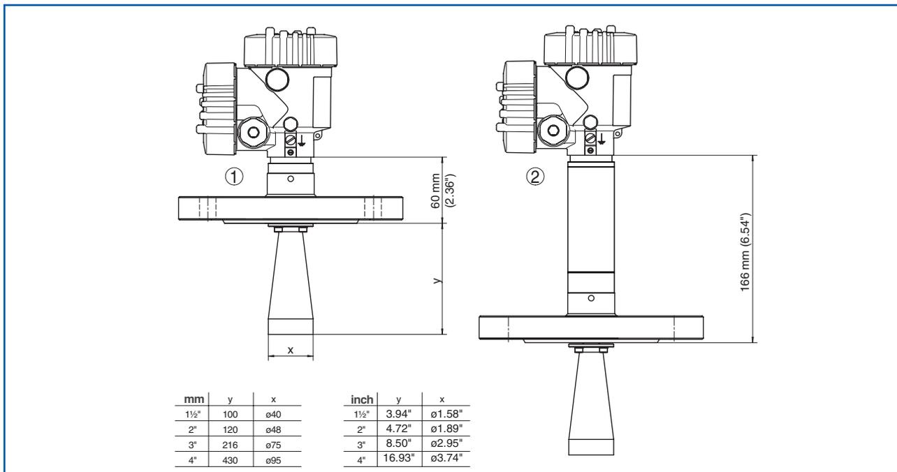
Fig. 41: Nico 30, horn antenna in flange design
