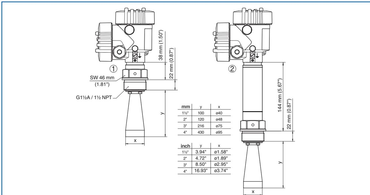
Fig. 40: Nico 30, horn antenna in threaded design
