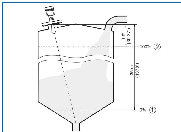
Fig. 35: Parameterisation example for Min. / Max. adjustment
