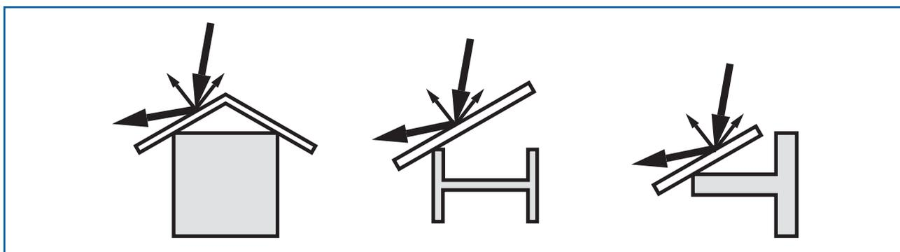
Fig. 21: Cover smooth sections with plates to scatter the signal
