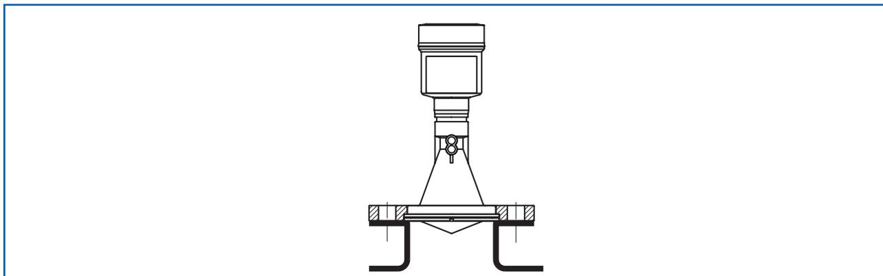
Fig. 14: Recommended pipe socket installation
