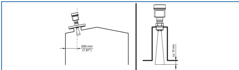
Fig. 1: Distances between the antenna and the vessel wall / roof
