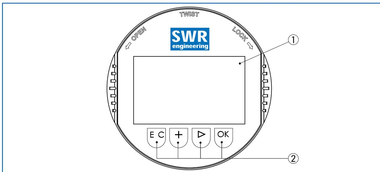
Fig. 34: Display and control elements
