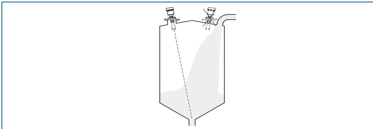
Fig. 12: Radar sensor installation with inflowing solids
