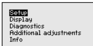
**Setup:** Settings, for example measuring point name, application, vessel, adjustment and signal output
