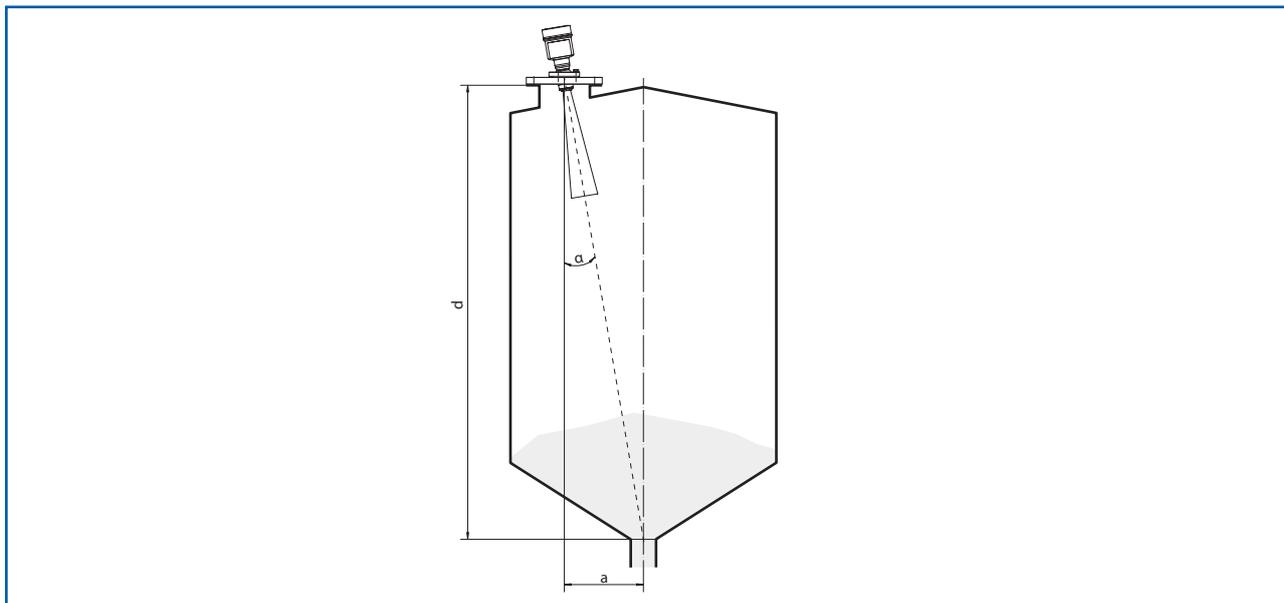
Fig. 20: Suggestion for installation after alignment of the Nico 30
