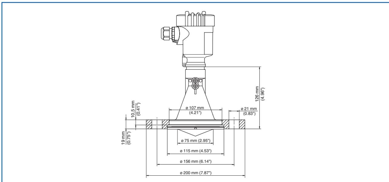
Fig. 38: Nico 15, collar flange to match DN 80 PN 16 / ASME 3" 150lbs/JIS80 10K
