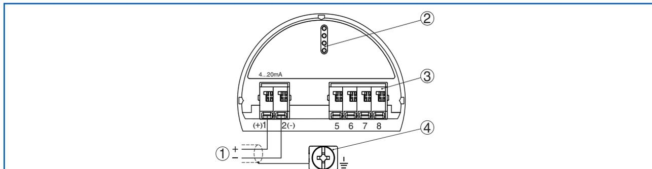
Fig. 31: Electronic and connection chamber in single-chamber housing
