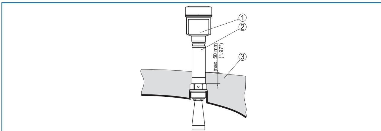
Fig. 24: Device installation on insulated vessels
